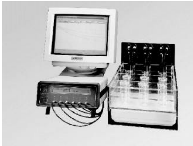
Figure 6 The Strathkelvin Activated Sludge Respirometer which utilises 6 oxygen electrodes connected via an interface to the pc loaded with dedicated respirometry software.
