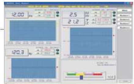
Modbus Realtime Data Display
