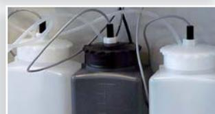
Continuous monitoring of reagents using level probes. The DPD reagent in powder form (to be diluted before use) is an excellent solution for safe storage.
